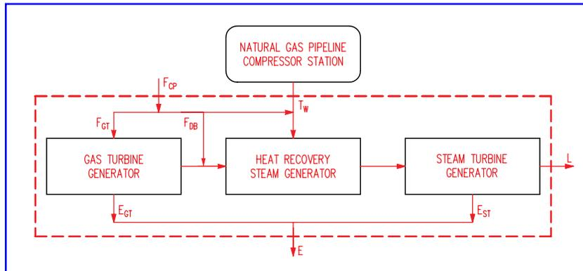
**Figure 2.1.3 Enhanced Combined Cycle System Energy Balance**
