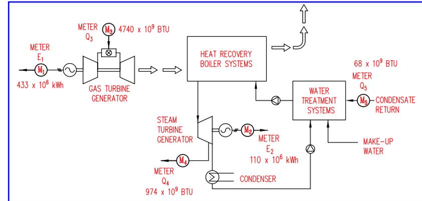
Figure 2.1.2 Natural Gas-Fired Combined Cycle in Cogeneration Mode
